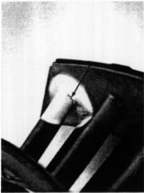
Figure HGP-I.3. Nozzle Partition Fillet Cracks.
